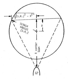
$$\frac{H}{2} \left( \frac{1}{2} \right) = \frac{\Delta \text{ OEFF R SCAN}}{2 \text{ (SIN } \phi) \dot{x}} = \text{TIME FOR ONE-WAY SCAN} = 2 \left( \frac{1}{\dot{\beta}}_{MAX} \right)_{TAN} - 1 \left[ \sqrt{\frac{S.R.^2 - \chi^2}{R \text{ CENTER}}} \right]$$
